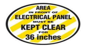
Make sure there is sufficient clearance to operate and service electrical equipment safely. The chance that a worker may be shocked increases when he or she works on equipment with energized and exposed parts in a cramped space. Because of the danger posed to workers who work in cramped spaces, Cal/OSHA has established regulations setting minimum clearances around electrical equipment rated at 600 volts or less. The minimum clearances depend on:
