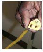
Should the ungrounded frame of a hand tool becomes energized, the quickest and easiest path for the current to take to ground is through the worker. Depending on the conditions, the severity of the shock will range from slight to fatal.
