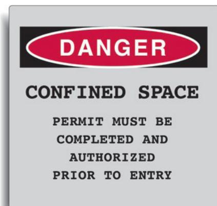
Examples of confined spaces include: water and sewer pipes, pumping stations, manholes, boilers, vats, kilns, vaults, silos, storage bins, meter vaults, tunnels, tanks, wastewater wet wells, grit chambers, utility tunnels, crawl spaces under floors, water reservoirs, holding tanks, pits, and sumps.
