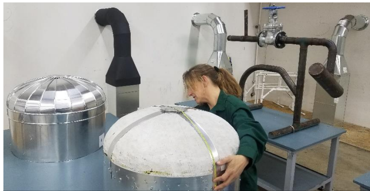
Veronica measures a tank head before creating a metal layout.
