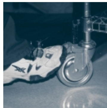
▲ Jammed wheel, faulty brake
